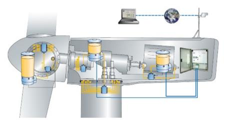
Typical components subject to friction and wear in wind turbines (SKF. Realize the lubrication potential for your wind turbines. Retrieved from https://www.skf.com/de/industries/wind-energy/operation-and-maintenance/windlub
